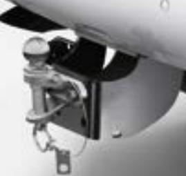
Toyota towing hitches are available with a flanged, fixed or detachable hook. Each provides a strong towing capability and will support the Toyota clamp mounted rear bicycle holder.
